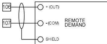
In some cases it may be desirable to place an isolating signal conditioner in the remote demand signal between the source and the Boiler Manager. The diagram below shows a typical connection of this type.
