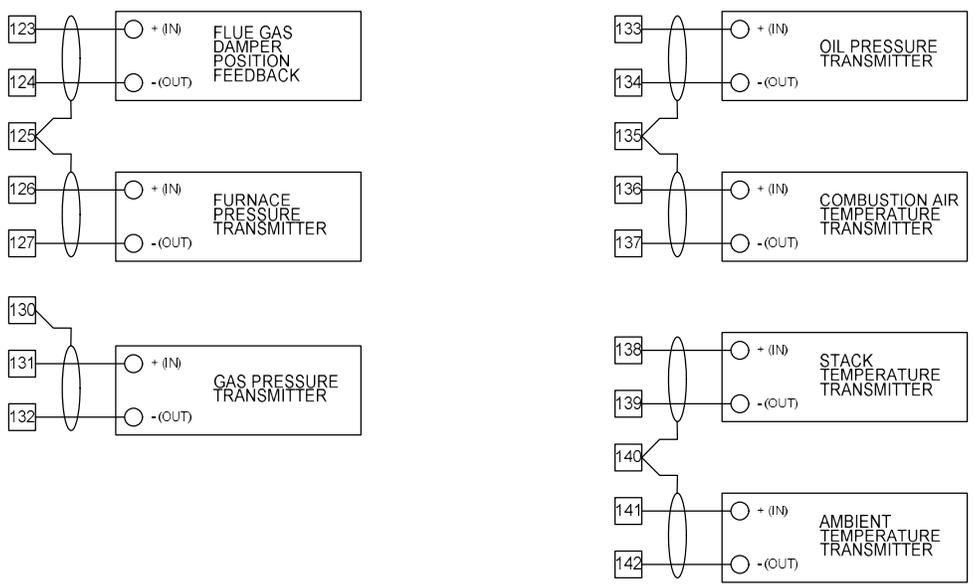
Any where that a transmitter is not used for a specific boiler installation, the “input” terminal should be connected to the 24VDC common (terminal 102) using a jumper wire. This will help reduce noise into the system from unconnected inputs.
