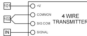
The diagram below shows terminal connections for all of the transmitters that the Boiler Manager accepts. Some of these may not be applicable on a specific boiler.
