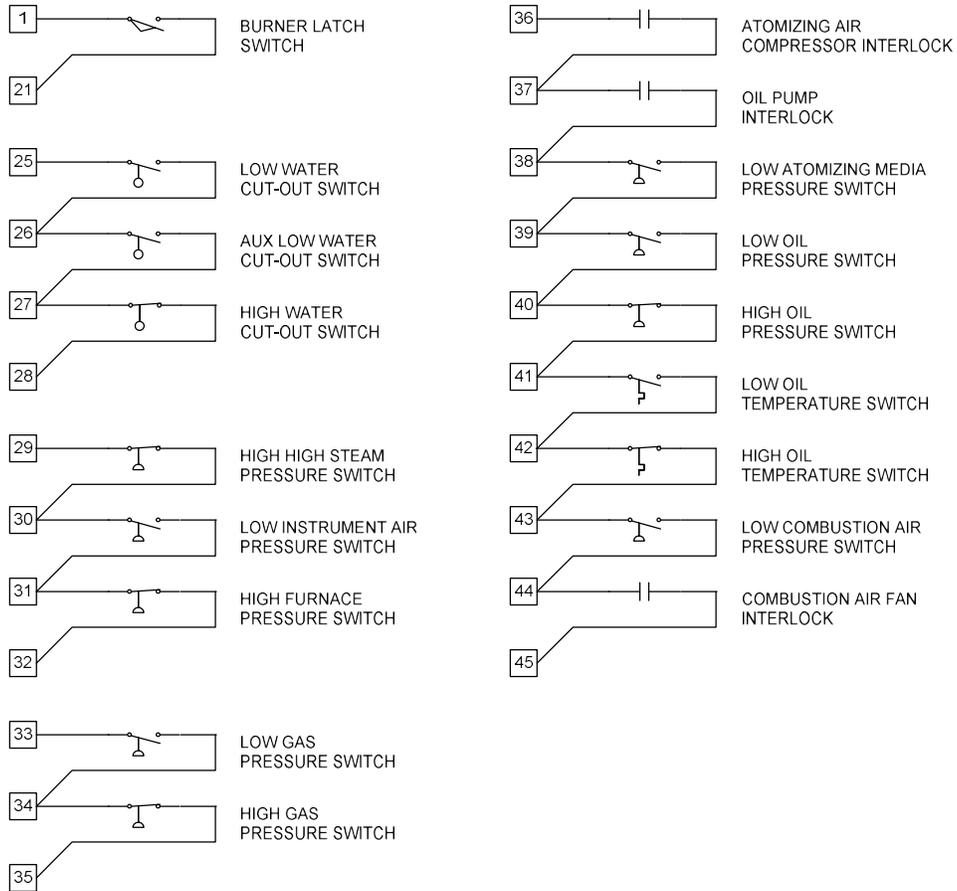
The remaining switches (that are not used to cause a safety shutdown) are wired to the terminals as shown below. Most of these switches are provided with a dedicated pair of terminals so that each terminal will only have one field wire connected to it.
